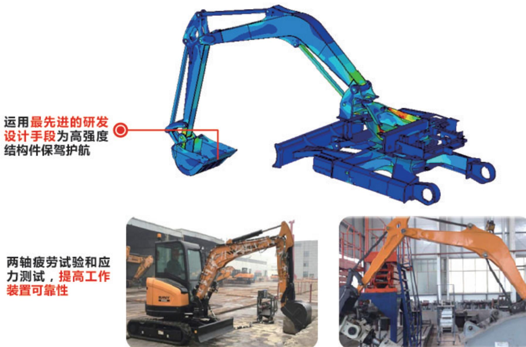
● 完备的研发试验体系 | Research and development of test system
